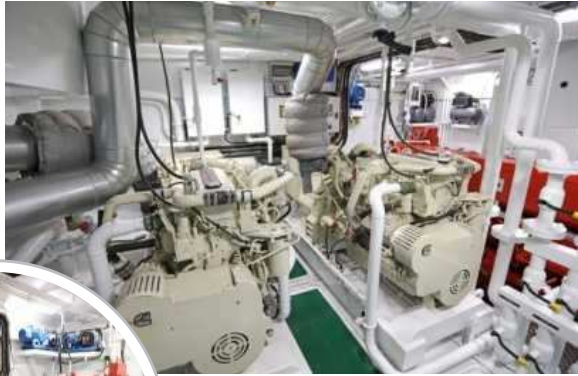
▲ Twin Cummins QSB 7 auxiliary engines drive 191kVA generators. ◀ The ABC 6DZ main engine.
