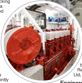
▲ Twin Cummins QSB 7 auxiliary engines drive 191kVA generators. ◀ The ABC 6DZ main engine.
