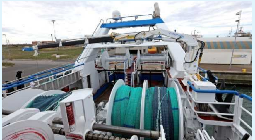
Looking aft along the trawl deck from boat deck level, showing some of the Rapp Marine deck machinery including the elevated single net drums positioned under the main trawl gantry; split nets drums forward on the trawl deck; split trawl winches and the Toimil 20t/m folding deck crane.
